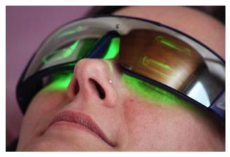
A Light and Sound machine is made up of a little small box like a mobile phone with headphones and light frames attached. And the light frames are literally a pair of sunglasses with LEDs embedded into the lenses. You put on the light frames and the headphones and you close your eyes and you keep your eyes closed.
